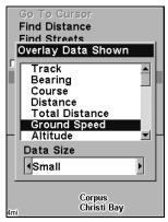
Overlay Data command on the GPS Menu, at left. Overlay Data Shown selection menu, right. In this example, we scrolled down the data list to highlight "Ground Speed."
